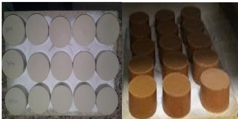
Figure 1 Shaped samples (75 bar) and Sintered samples (at 1000 °C)
